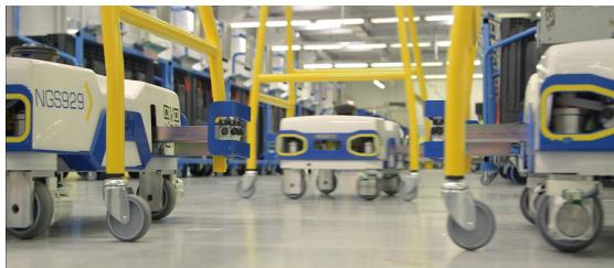
In these last months, we have also put into operation a trial configuration of **Soly™** in Bologna. Soly™-SORT, the SOLYSTIC product based on mobile robots enables automatic parcel sorting without fixed infrastructure and definitely removing any need of weight lifting by operator.
