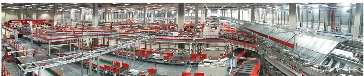
The new, forward-looking hub of bpost (Belgium postal operator), which will open its doors in 2017 in the Brussels area, is a good example of this growing importance of IT. A "Multisorting Parcel Handling System" (MPHS) supplied by Italian company Leonardo (900 meters long and handling more than 30,000 parcels per hour) is currently being integrated with the IT system supplied by SOLYSTIC, already in operation in the country for mail processing.
