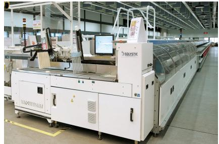
The solution is based on the SOLYSTIC XMS™ product, widely adopted by many postal operators, which sorts and prepares the delivery for both "letter" and "flat" mail (large envelopes, magazines, plastic wrapped items).
